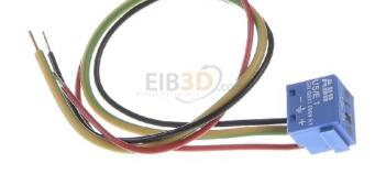
Surge protection for signal systems Nominal discharge surge current (8/20) 5kA, Nominal load current 6A, Voltage protection level core/core 750V, Voltage protection level core/earth 500V, Mounting method Connector/cable adapter, Connection 1 Clamp, Signalling at the device None
