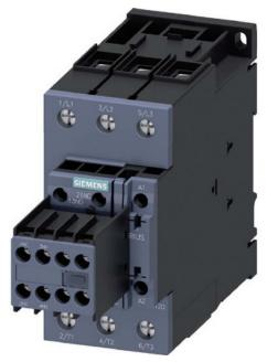
Contactor 22kW/400V, 1NO+1NC - Magnet contactor 51A 100VAC 3RT2036-1AG64
