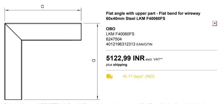
Flat bracket with upper part LKM F40060FS Height 40mm, width 60mm, version lower part and upper part, angle 90 ... 90°, material steel, surface galvanized, color other, type of fastening bottom perforation, flat bracket with upper part for changing the direction of the cable routing ducts LKM. Equipotential bonding is guaranteed between the lower and upper parts without any further aids.
