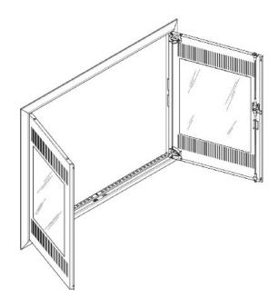
Blind frame with media door for UP-VT, 4x5 rows - Door for cabinet 1050mmx800mm steel GBRU45TM
