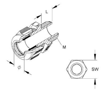
IPON cable gland M16, for cables 3, 5-10 - Cable gland / core connector M16 1234ML1601
