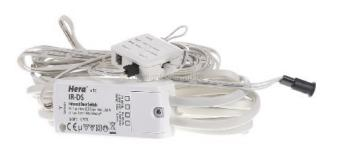
IR door contact switch 50612080242 basic element, non-contact door contact switch for connecting lamp operating devices of protection class II, mains connection cable 3m and switching cable 0.3m, each stripped and with ferrules for easy connection to screw or plug-in terminals, sensor cable 3m with sensor head K60, switching function: The light switches on when the door is opened and off again when the door is closed, including automatic safety switch-off of the lights after 30 minutes
