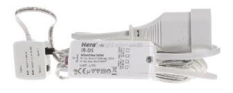
IR double contact switch 50612090221 base element, non-contact door contact switch for connecting lamp operating devices of protection class II, 3 m connection cable with Euro plug, 0.3 m switching cable with Euro coupling, two 3 m sensor cables with K60 sensor head, switching function: when one of the two is opened Doors, the light switches on and off again when both doors are closed, including automatic safety switch-off of the lights after 30 minutes
