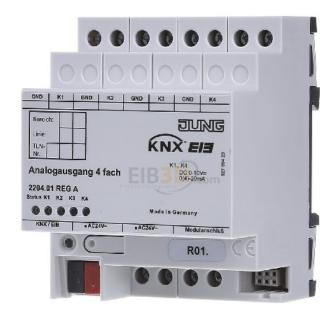
KNX analogue actuator 4-fold for the conversion of KNX telegrams to analogue signals 2204.01 REG A
