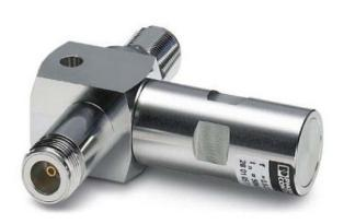
Surge protection device N connectors female/female CN-LAMBDA/4-2.25-BB Rated discharge surge current (8/20) 50kA, rated load current 5A, protection level wire/earth 5V, frequency 800 ... 2250MHz, other type of installation, connection 1 N connector , Signaling on the device without, adapter plug with Lambda/4 technology as surge protection for coaxial signal interfaces. Connection: N connectors socket-socket
