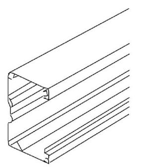
Trunking base, pure white, spandrel trunking - Wall duct 105x66mm RAL9010 BU651058.3
