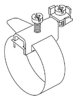
Grounding band clamp with connection ring - Earthing pipe clamp 17,5...48mm 37/1
