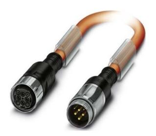
Connector plastic-coated on both sides - Power cable < 1kV, moving inst. K-5E-M40 M9/#1620380
