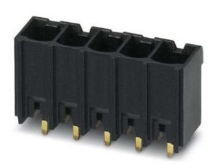
Socket insert VS-MSTBAH 2,1657915 number of poles 5, connector insert material thermoplastic, rated current In 16A, ambient temperature -40 ... 70°C, rated voltage 24V, contact coating material other, contact insert material other, contact material other copper alloys, flammability class of the insulating material according to UL 94 V0, MSTB contact insert, for printed circuit board mounting, 24 V, 5-pin, with angled solder pins, RAL 9005 (black), for mounting frame VS-PPC-F2-MSTB-...-1R-P
