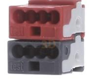
Bus terminal 2p.4 plug-in connection. 5WG1193-8AB01 KNX bus system, other bus systems without, bus connection terminal design, instabus EIB bus terminal 193, 2-pole 4 plug-in connections red/dark grey
