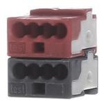
Bus connection terminal 689701 Bus system KNX, Other bus systems without, Bus connection terminal design, For connecting a maximum of 4 wire pairs to a KNX device, can also be used as branch terminal. Consisting of two latched terminal parts, red (+) and dark gray (-), each with 4 plug-in terminals. For solid conductors with a diameter of 0.6 to 0.8 mm. Colour: red/dark grey.
