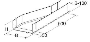
Cable tray height 80 mm, Width (large dimension) 500 mm, Width (small dimension) 100 mm, Design Reduction to the right, Execution integrated connector, Wide span execution no, Suitable for function maintenance no, Material Plastic, Stainless steel, stained no, Material quality GFK, Surface protection other, Colour other, RAL-number 7032
