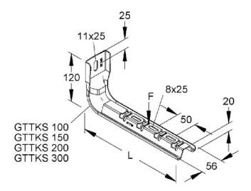
Hanging support and wall bracket 120x215mm 1.08kN - Wall- and profile console GTTKS 150 S
