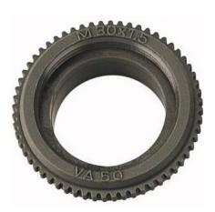
Valve adapter VA50 639150 Type of accessory others, for Honeywell+Braukmann, Reich, Landis+Gyr, MNG, Cazzagniga. Valve adapter for adapting to different valve bodies and heating circuit distributors. To be completed with: Thermoelectric actuator 230V 639125. Thermoelectric actuator 24V 639126.
