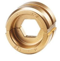
Press insert 70qmm D 22/70 Application compression cable lugs and connectors, cross-section 70 ... 70mm², hexagonal compression (hexagonal), suitable for compression cable lugs (DIN 46235) and connectors (DIN 46267, Part 1) according to DIN - Cu.
