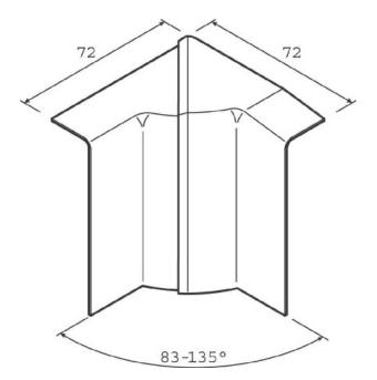
Inside corner VDI - Inner elbow for baseboard wireway SL 200804 gsw
