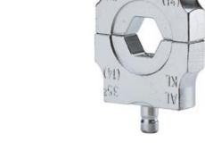
Crimping insert HA 4/70 Application compression cable lugs and connectors, cross-section 70 ... 70mm², hexagonal compression (hexagonal), suitable for compression cable lugs and connectors according to DIN - AI, compression cable lugs and connectors AI/Cu (aluminium side).
