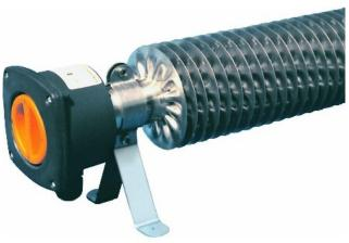
Finned tube heater 230V, 2000W, 1100mm RRH ST 2000 power 2000W, fin diameter 120mm, voltage 230V, protection class (IP) IP67, height 184mm, width 145mm, length 1100mm, finned tube heater with 3-stage switch, finned tube and mounting feet made of stainless steel material no. 1.4512, connection box made of glass fiber reinforced polyamide.
