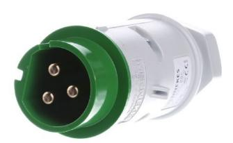
Plug 32A,3p,4h 677A IEC current 32A, UL/CSA current (if UL version desired) 30A, number of poles 3, voltage according to EN 60309-2 20-25 V / 40-50 V (100-200 Hz) green, time position 4h, code color green, RAL number 6010, degree of protection (IP) IP44, connection technology screw terminal, cable entry anti-kink sleeve, plug-in direction straight, material plastic, plug, 32A3p4h, low voltage, IP44 with screw connection
