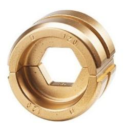
Press insert 6qmm D 22/6 Application compression cable lugs and connectors, cross-section 6 ... 6mm², AWG range 10 ... 10, hexagonal compression (hexagonal), suitable for compression cable lugs (DIN 46235) and connectors (DIN 46267, Part 1) according to DIN - Cu.
