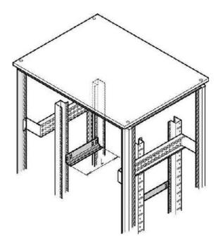
Slide rail 1 pair, 800T - Accessory for switchgear cabinet 22127094 (VE2)
