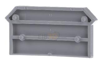
End/partition plate for terminal block Type of end plate, Type of partition, Colour Grey, Thickness 4mm, Snap in, Inflammability class of insulation material acc. with UL94 V0
