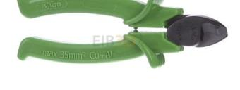
Mechanic one hand shears, Type/operation mechanically one-handed, Max. cable cross-section 35 mm², Suitable for stranded conductors yes, Suitable for fine-wire conductors yes, Suitable for solid conductors yes, Suitable for steel wire braiding no, Cutting head replaceable no, Cutting jaws interchangeable no, With stripping function no, Insulated yes, Protective insulation 1000 V no, Handle version 2 components, VDE tested yes, With impact protection no
