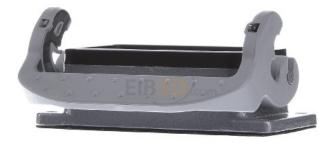
Width 43.5 mm, Height 28 mm, Execution of the housing Mounted housing, Material of the housing Aluminum, Housing Color gray, Arrangement of the cable feed other, With cable gland no, With hinged lid no, Type of lock Locking latch, Operating temperatur -40..120 °C, EMC version no, Corrosion resistant yes, UV-resistant yes, Degree of protection (IP), mounted IP54
