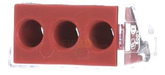
Socket clamp 3x2.5-6qmm, transparent 773-173 Number of clamping points 3, nominal cross-section 2.5 ... 6mm², color transparent, nominal voltage 400V, nominal current 41A, suitable for solid conductors, suitable for stranded conductors, solid conductor cross-section (solid/stranded) 2.5 ... 6mm², AWG range 14 ... 10, junction box terminal for solid and stranded conductors max. 6 mm² 3 conductors Housing color transparent Cover color red Ambient temperature max. 60°C
