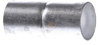
Aluminum push-fit socket AMS-E 25 Material metal, material quality aluminium, surface untreated, quality of the surface coating uncoated, halogen-free, plug-in version, for nominal pipe diameter 25mm, color natural, material of the seal without seal, AMS-E is an aluminum push-fit socket made of extruded Aluminum. This sleeve is used to connect the aluminum tube Alu Steck-ES. VDE 0605 DIN EN 61386-21
