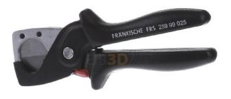
Ergonomic pipe cutter FRS 25999025 Suitable for plastic, pipe diameter 12 ... 25mm, length 185mm, FRS is a pipe cutter with blade made of high-strength special steel, hardened and tempered in oil. The ergonomically shaped handles are made of glass fiber reinforced plastic. The scissors are used for the exact right-angled cutting of plastic pipes in a diameter range of 12 - 25 mm. The advantages lie in clean, smooth and burr-free cut surfaces. Not suitable for cutting cables.
