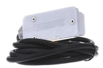
Sun sensor 9050100 Brightness sensor version, sun sensor/sensor for animeo IB+, MC2, SM 2000 slide switch, without mounting bracket, for direct connection to the Outside Sensor Box, W x H x D 34x88x47 mm, IP 65
